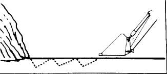
It is important to keep the bucket level when approaching a bank or pile. This will help prevent gouging the work area.
